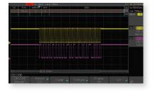
Protocol Trigger and Decode – The T3DSO1000 displays the waveform decoding and events list. Bus protocol information can be quickly and intuitively triggered and displayed.
